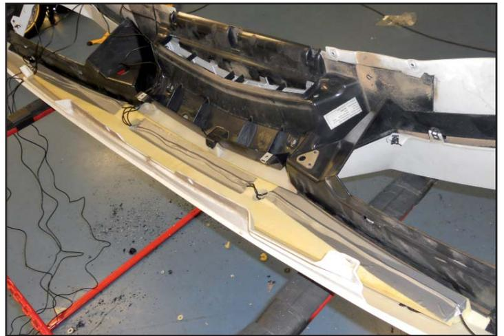
Also take down the polyurethane vibration-damper support.
