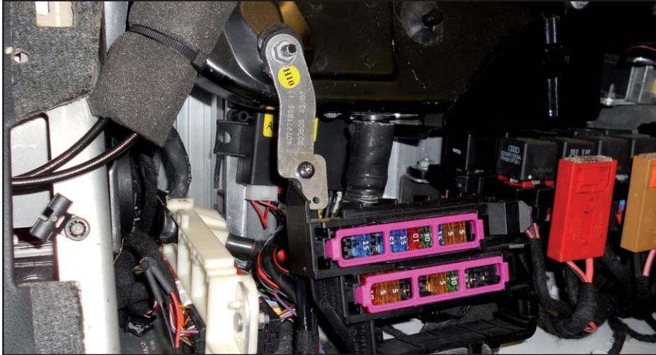
The front management control unit and the CAN BUS utility module must be set up over the GFA control unit located under the glove compartment, on the passenger's side.
